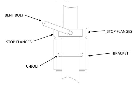
**CAUTION:** TO AVOID TIPPING OF THE HEATER. THE LONG CENTER LEG MUST BE ALIGNED WITH THE ARROW ON THE BRACKET, THE BENT BOLT ALIGNED WITH THE ARROW ON THE CURVED PLATE, AND THE BENT BOLT CAPTURED BETWEEN THE STOP FLANGES!
